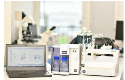
The Ampha Z32 Impedance Flow Cytometer set up in the Lab with the autosampler and a laptop showing measurement results.
