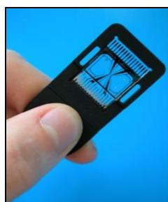
Fig. 2 Impedance micro-fluidic chip in holder frame.
